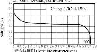
寿命特征图 Cycle life characteristics Discharge capacity (min)
