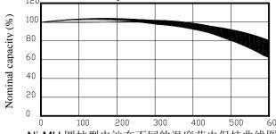
Ni-MH 圆柱型电池在不同的温度荷电保持曲线图 Charge retention curves of Ni-MH cylindrical cell At various storage temperature
